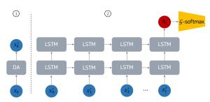
Figure 4: The 2SRNN architecture: 1) DA component, 2) Sequence classifier.
