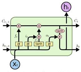
Figure 3: LSTM cell architecture (Olah, 2015).
