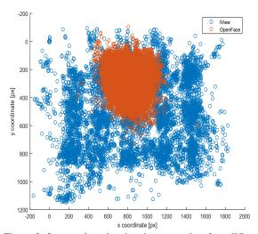
Figure 5: Scatter plots showing the output data from iView and OpenFace. It is shown that the output from the Open-Face is concentrated in the certain area of the the screen.
