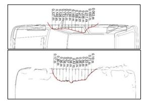
Figure 14: Skoda Felicia side impact – top-view (up) vs. scanner (down).
