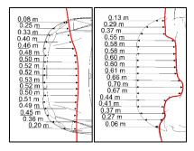
Figure 6: Fiat Multipla frontal impact – top-view (left) vs. scanner (right).
