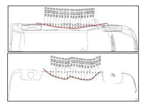
Figure 12: Chrysler Voyager side impact – top-view (up) vs. scanner (down).
