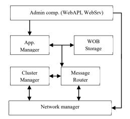
Figure 3: Middleware internal structure.
