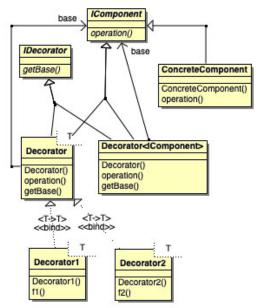
Figure 5: The Class Diagram of the HybridDecorator Pattern - The General Solution.
