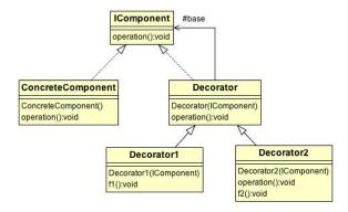
Figure 1: The Class Diagram of the Classical decorator Pattern.
