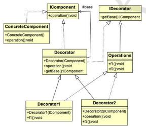
Figure 2: The Class Diagram of the MixDecorator Pattern.
