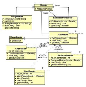
Figure 4: The Class Diagram of the HybridDecorator Pattern Applied to the *Reader* Problem.
