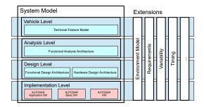
Figure 1: EAST-ADL abstraction levels with the containing models and extensions (based on (Blom et al., 2016)).
