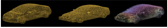
Figure 4: From left to right: the template, a car shape, and the flow for mapping them.
