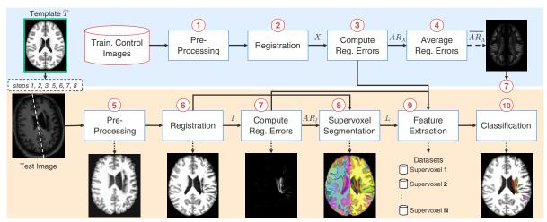
Figure 2: Pipeline of BADRESC. The upper blue part is computed previously (offline). The bottom orange part is computed for each test image. The template (reference image) is used in both parts (Steps 1, 2, 3, 5, 6, 7, and 8). Figure based on (Martins et al., 2019b; Martins et al., 2019c).
