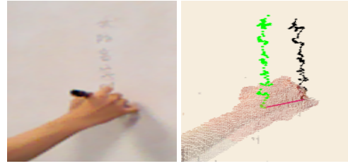
Figure 4: For the chinese writing style on the whiteboard, shown in the right picture, the 3D hand's centroids (the green points) are projected onto the plane (black points on the orange background). The red line represents the vector parallel to the plane normal projecting the current centroid onto the plane.
