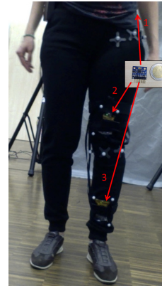
Figure 2: The red arrows show three IMUs which are mounted on 1.pelvis (not visible), 2.upper leg and 3.lower leg.
