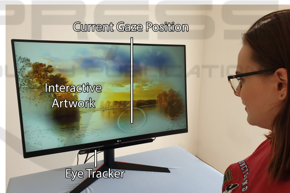
Figure 1: A user interacting with the system. The eye tracker, mounted at the bottom-side of the monitor, records the eye movement of the user. On the connected computer, the application displays the computer-generated artwork, which is influenced by the processed sensor inputs.
