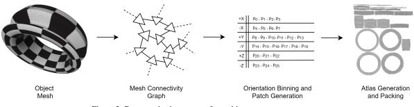
Figure 3: Parameterisation process from object space to texture space.
