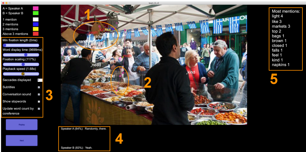
Figure 5: Overview of the prototype. 1: Fixations and words spoken by a participant while looking in the surrounding area. 2: Fixations and saccades in different colors corresponding to a speaker. 3: Various settings. 4: Machine-transcribed subtitles of the dialogue. 5: Words that are mentioned frequently displayed along with their frequency count.
