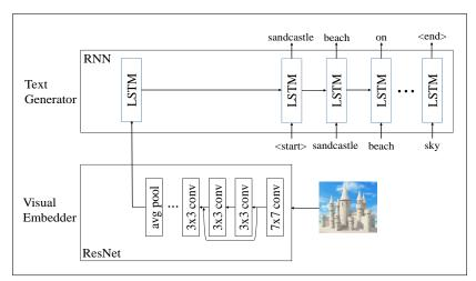
Figure 1: Neural model architecture: ResNet, a deep convolutional neural network is used to create a semantic representation of an image, which we then decode using an LSTM network. The vectorized image representation is fed into the network, followed by a special start-of-sentence token. The hidden state produced is then used by the LSTM to predict or generate the caption for the given image word-embeddings.
