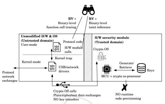
Figure 2: RV-centric comprehensive security for cryptographic protocol implementations (USB stick example).
