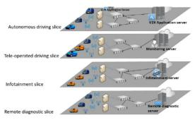
Figure 3: General architecture of network slicing.
