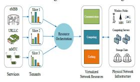
Figure 5: 1 Slicing in next-generation wireless networks (NGWNs) (Alcardo Alex Barakabitze, et al., 2019).
