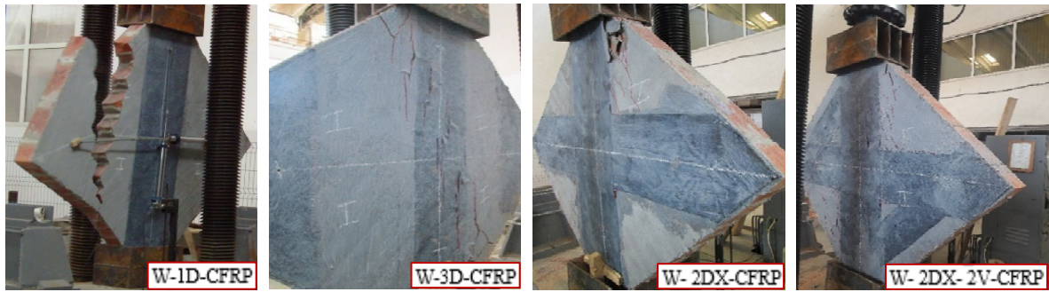
Wall shear cracking (Group N°2)
