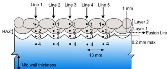
Figure 3: Specific test location points of specimen 2 based on Aramco Drawing AB-036386.
