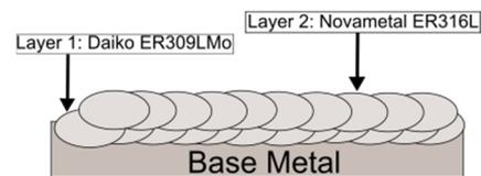
Figure 1: Weld overlay layout.
