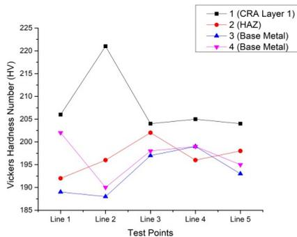
Figure 4: Graphical representation of specimen 1 measured Vickers hardness number (HV).
