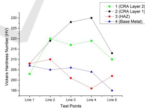
Figure 5: Graphical representation of specimen 2 measured Vickers hardness number (HV).
