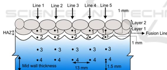
Figure 2: Specific test location points of specimen 1 based on API 5LD specification for CRA Clad or Lined Steel Pipe.
