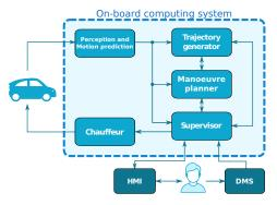
Figure 1: Autonomous driving architecture for Autopia Program.
