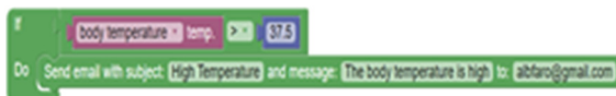
Figure 10: Blockly program to send an alert when the body temperature is higher than 37,5 °C.
