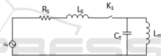
Figure 1: Operation circuit breaker overvoltage equivalent circuit diagram.
