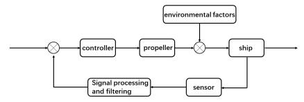
Figure 1: The structural diagram of the ship's dynamic positioning system.
