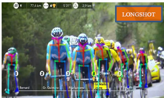
Figure 5: Results of pose detection and shot type estimation on a Tour de France 2019 broadcast.
