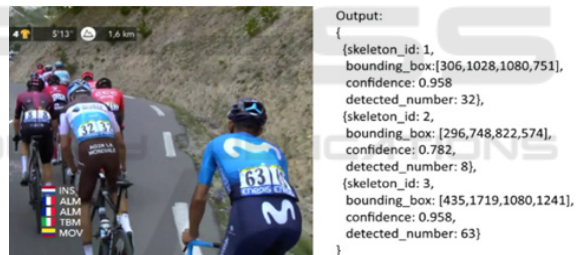
Figure 9: Results of number recognition algorithm.
