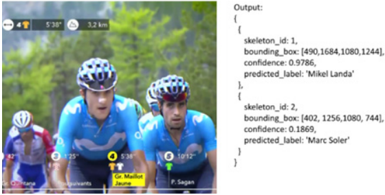
Figure 10: Results of face recognition algorithm.
