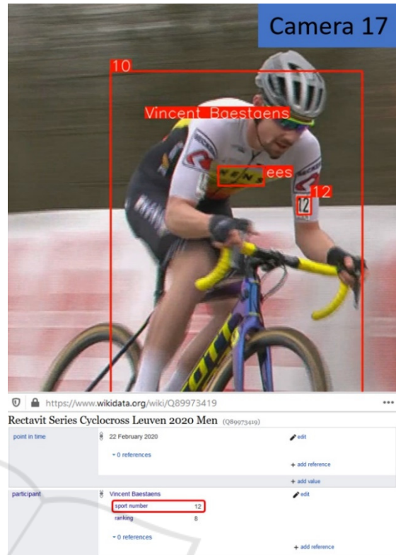
Figure 10: Example of optical character recognition (OCR) on camera 17 output stream. With the combination of the detected shoulder number and the participant list added to the race’s WikiData page the rider was correctly recognized. In combination with the camera proximity algorithm this can produce an accurate rider detector and tracker.
