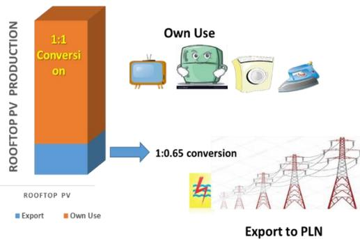
Figure 4: Illustration of Rooftop PV Production of kWh Calculation.
