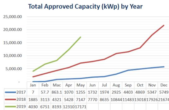
Figure 5: Total Approved PV Capacity (kWp) by Year in Malaysia.
