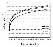
Figure 2: Correlation Between Presssure and Boiling Point
