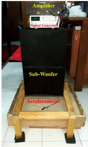
Figure 9: The prototype of the buried object detection system.
