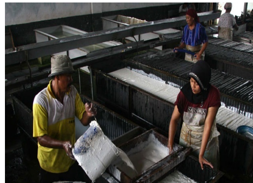
Figure 1. Workers not using PPE
