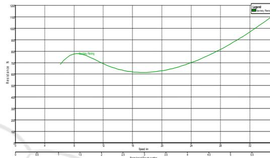
Figure 5: Resistance v Speed Curve
