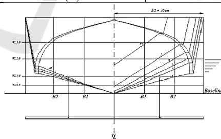
Figure 1: Body Plan of Hydrofoil Craft
