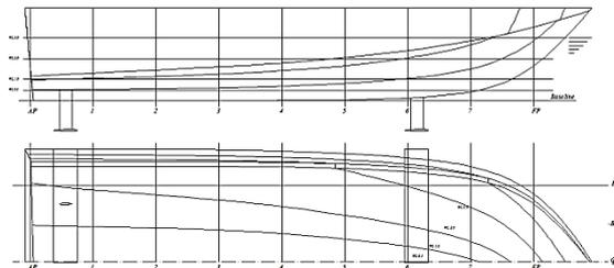
Figure 2: Profile and Plan View of Lines Plan
