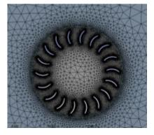
Figure 3. The meshing pattern of the turbine
