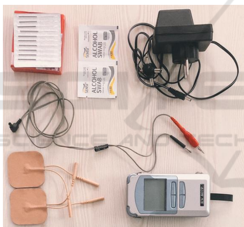
Figure 1: A modified electrical stimulation device (Everyway EV-807P NMES).
