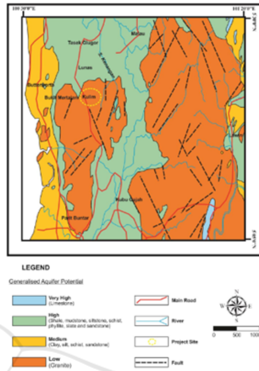
Figure 3: Geological Map of the study area, which consists of granite and is surrounded by sedimentary rock and metamorphic rock (Hutchison, 1989).
