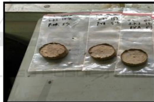
Figure 3: Porous ceramics with particle size oil palm stem powder a) 100 b) 150 c) 200 mesh.
