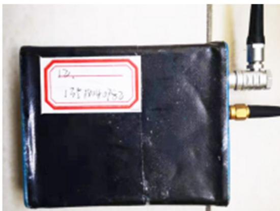
Fig 1. On-board data acquisition terminal.
