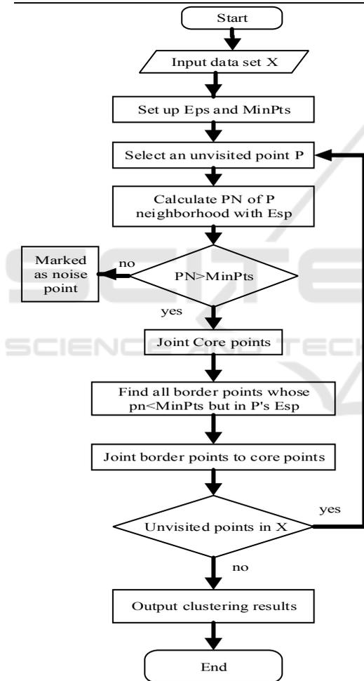
Fig 3. Process of DBSCAN clustering algorithm.
