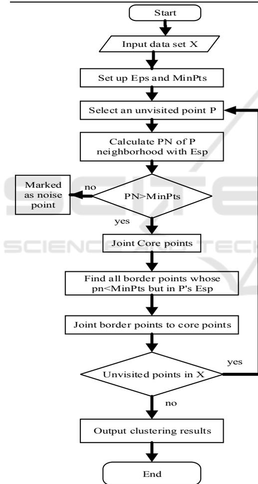
Fig 3. Process of DBSCAN clustering algorithm.
