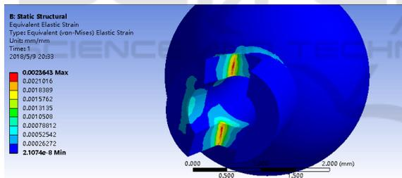
Figure 8. Nozzle deformation before improvement.
