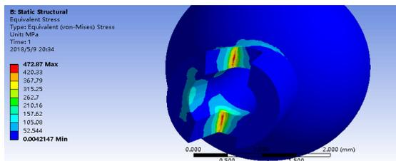
Figure 9. Nozzle equivalent stress cloud diagram before improvement.
