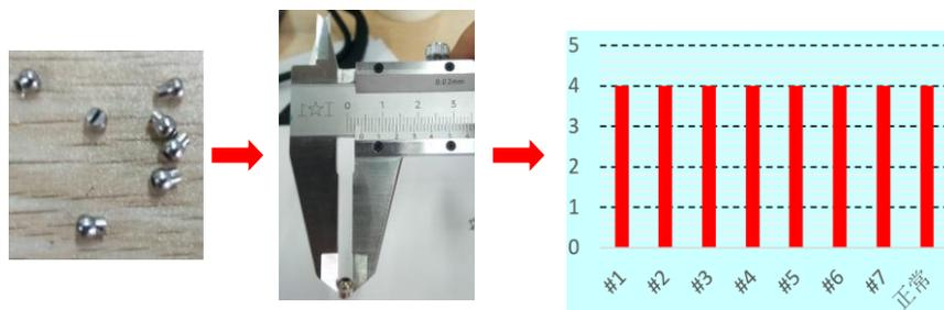
Figure 3. Nozzle ball head diameter measurement data.
