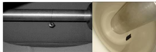
(a) Floating discharge defect (b) Surface discharge defect
