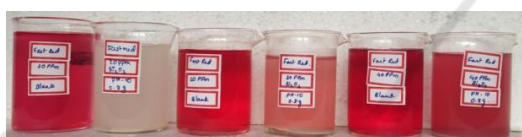
Photo 3. Effect of initial dye concentration on the photocatalytic degradation of Fast Red dye, Bi 2 O 3 g/pH=0.8/10
