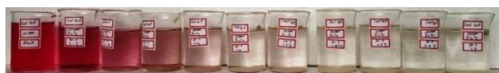
Photo 1. Effect of catalyst concentration on Fast Red dye at 120 minutes=20 ppm, pH=7
