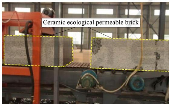
Figure 8. Ceramic ecological permeable brick.
