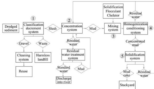
Figure 7. Sediment treatment system.
