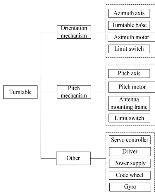
Figure 2. Overall block diagram of the servo system.
