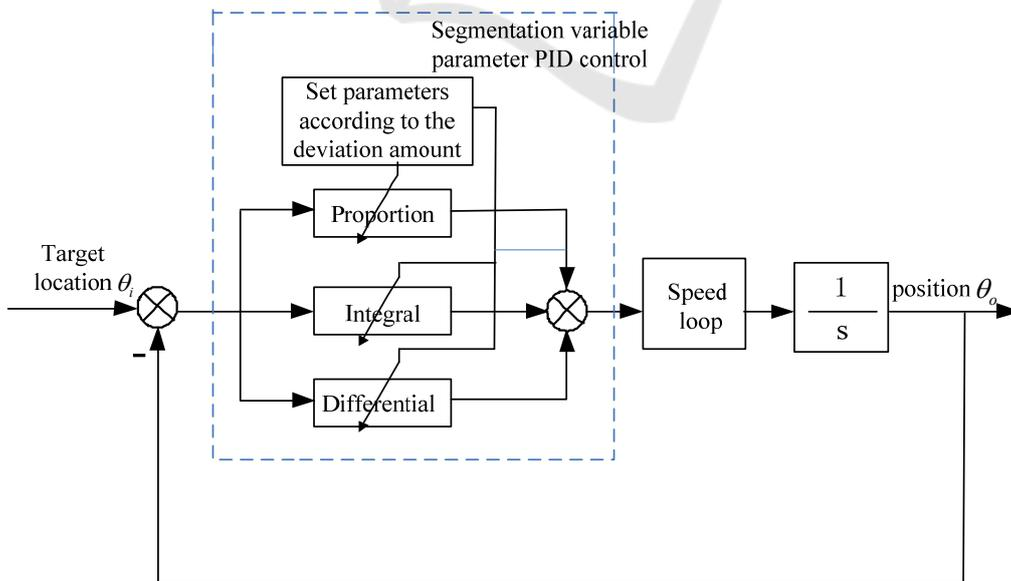
Figure 5. Schematic diagram of segmentation variable parameter PID control.
