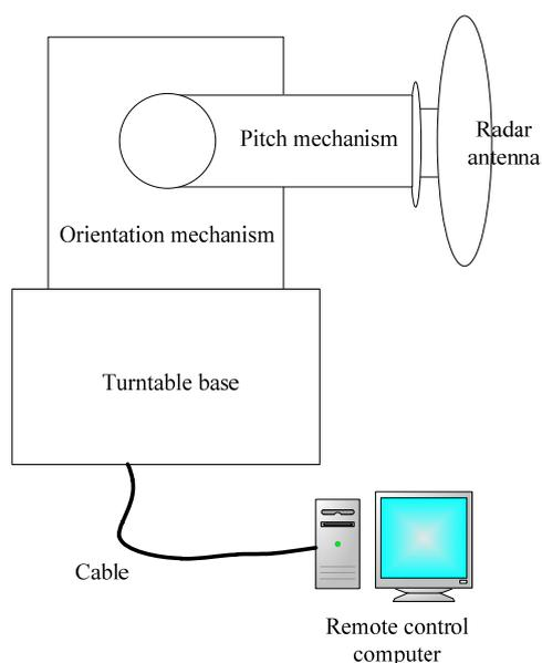
Figure 1. Block diagram of the stable platform.
