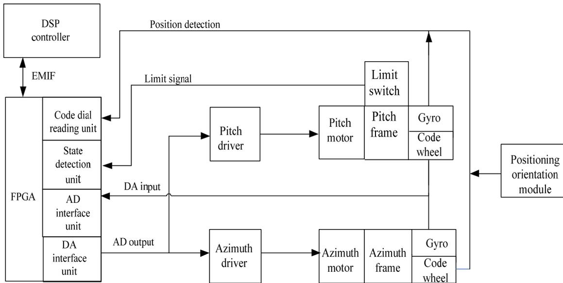
Figure 3. Schematic diagram of servo control circuit.
