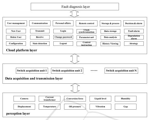
Figure 1. Structure of the fault diagnosis and PHM system for switch equipment.
