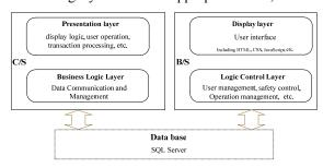
Figure 2. Software structure of the cloud platform.
