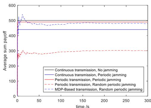
Figure 7: Comparison of different anti-jamming schemes.
