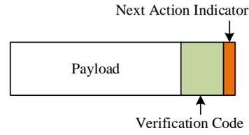
Figure 2: Component of a frame.
