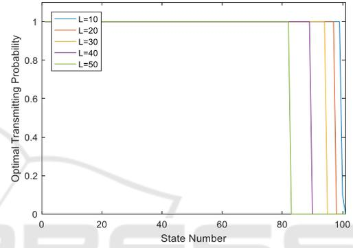
Figure 6: Optimal transmitting probability with different jamming loss with  $\sigma^2=0.1^2$ .
