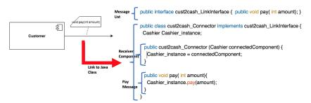
Figure 4: Transforming the link specification between customer and cashier components in Java and JML.
