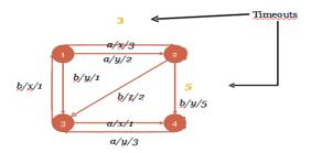
Figure 3: Finite state machine with timeouts.
