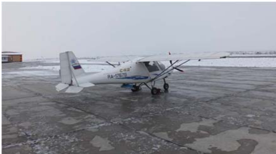
Figure 4: Flying laboratory, where computer vision system was tested to determine aircraft flight parameters based on visual data.
