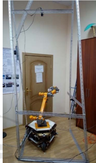
Figure 6: General view of test bench for controlling manipulator grip movements on movable base when performing complex manipulations (opening the door).
