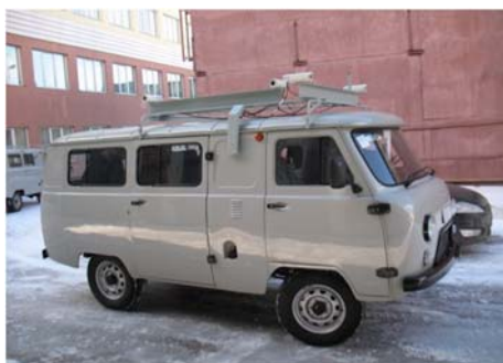
Figure 8: Two stereosystems installed on the mobile complex for operational mapping.
