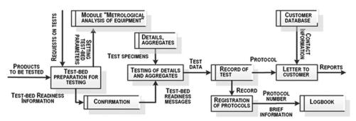
Figure 2: Diagram of data flows of the process "Testing of units and vehicle parts".
