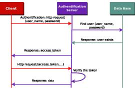
Figure 2: Token mechanism.
