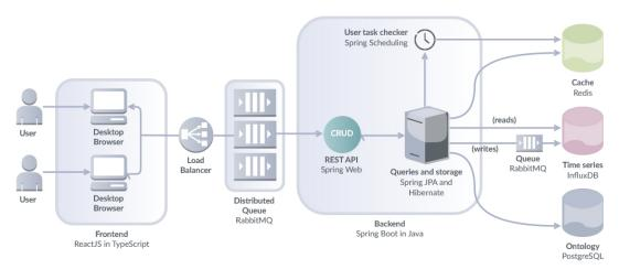
Figure 3: Platform architecture. The backend node can be replicated on-demand to accomodate intensive workloads.
