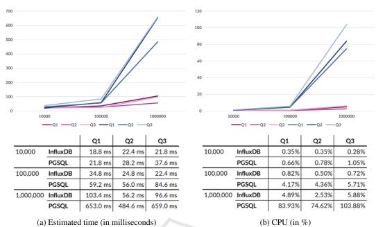
Figure 6: Average request time and CPU usage observed during reads. Purple lines are InfluxDB, blue lines are PostgreSQL.
