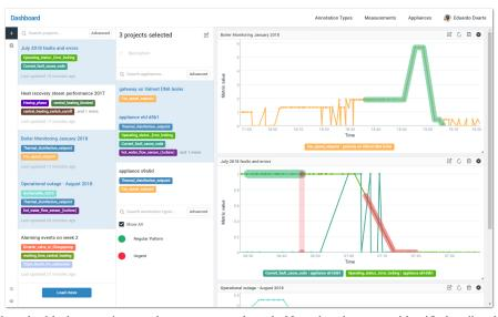
Figure 4: Dashboard with three projects and two sources selected. Note that the source identified as "appliance eb1d5b1" contains measurements from two separate projects, as these are merged when displayed on the source list.
