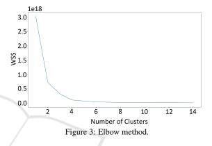
As shown, starting from four clusters, the distances of quadratic errors become approximately stable, showing that from that point, there is not a significant discrepancy in terms of variance. Therefore, the ideal number of clusters to this data set is four.
