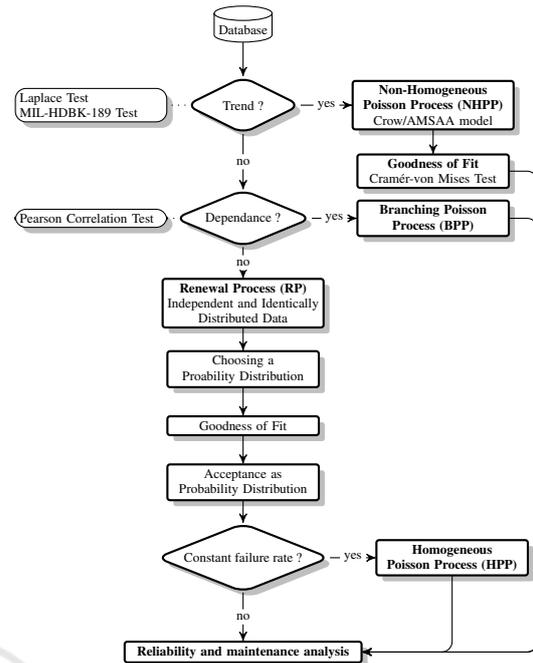
Figure 1: Reliability analysis process (adapted from Ascher and Feingold, 1984).
