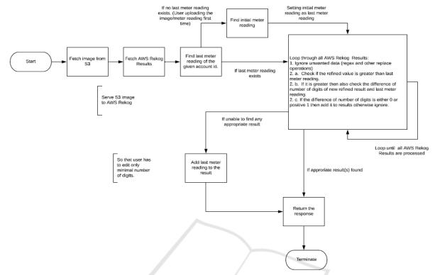
Figure 8: Results Refinement Algorithm for Image Recognition.
