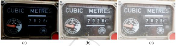
Figure 2: Gamma correction effect: (a) 0.25GAMMA, (b) 1.5GAMMA, (c) 3.0GAMMA.
